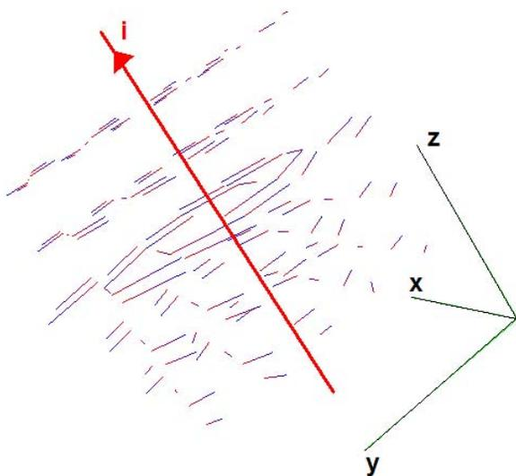
Figure 6: Linear current's reconstructed field.
