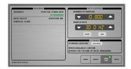
The user can adjust the clock at any time so is able to be synchronised to other equipment in the chain. Various data sets present on the storage device can be removed using the touch screen by touching on a session and deleting it. Data sessions are automatically named and no two will ever have the same name. Data is saved in a popular .CSV format and can be instantly converted into graph data without the need for tedious ASCII conversion and data collation.
