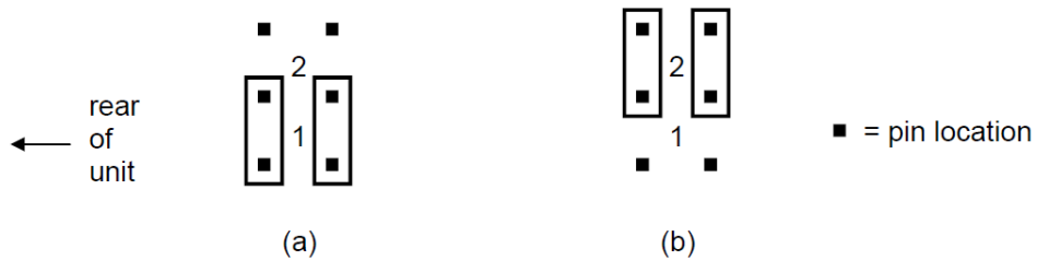
Fig. 4. Option Jumpers (a) Option 1 (b) Option 2
