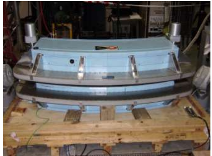
Fig. 4. Photo of retrofitted HTS coil dipole for VUV storage ring.
