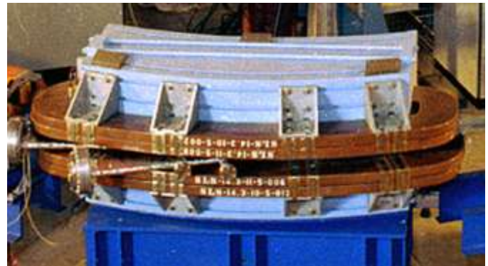
Fig. 3. Photo of copper coil dipole at NSLS.
