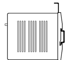
**Slide the DI downwards, so that the top edge of the DIN rail is hooked by the backplate.**
