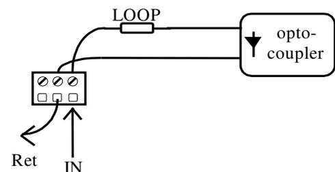
Each channel set to "LOOP" mode is isolated from all other channels.
