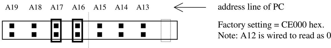
Hexadecimal coding table:    ■ = no jumper = 1    □ = jumper in place = 0
