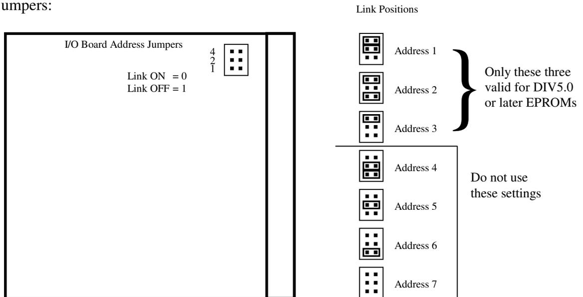
Note that early versions of the Type B board (PCB number 16000028A) and of the Type D boards (PCB number 16000029A) have board jumpers in a different position and/or orientation.
